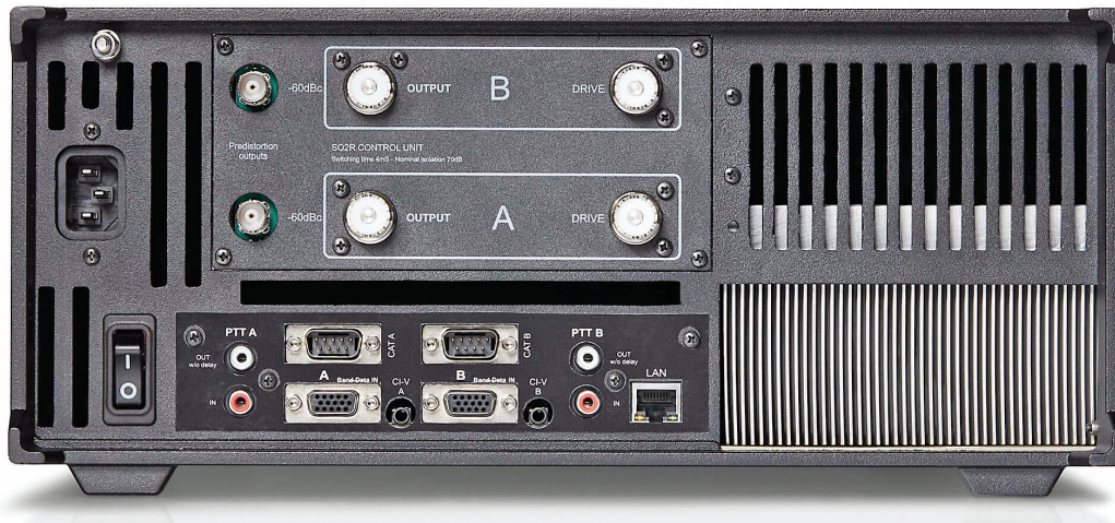
Figure 2 — The PGXL rear panel. RF input and output and predistortion sampler connections are in the upper center, with band data/CAT and PTT connections below. [Photo courtesy of FlexRadio Systems]
