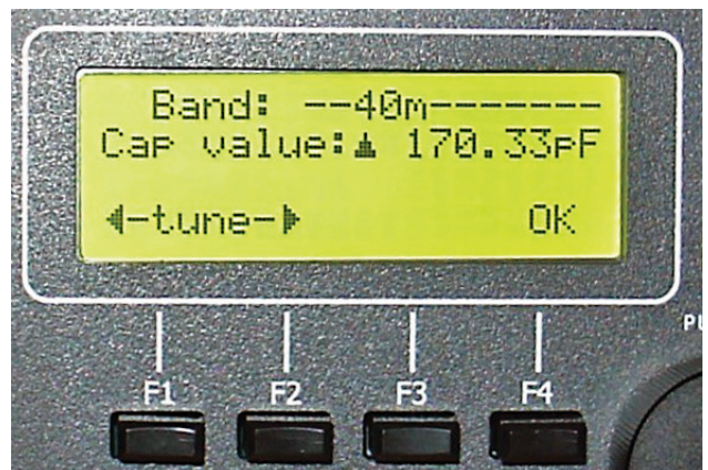
Figure 5 — Pressing BAND on the startup screen brings up this screen for changing to a different frequency band by using the arrow buttons ( F1 and F2 ).
