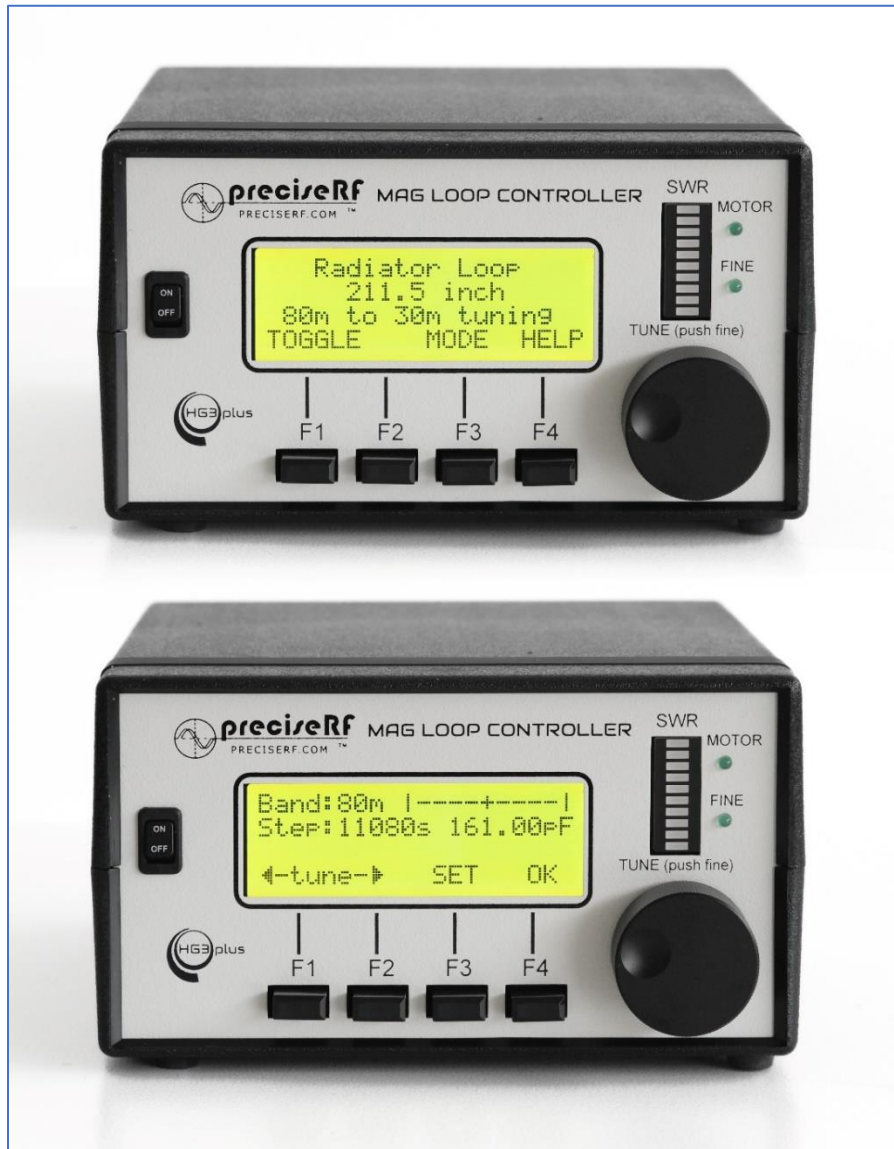
Figure 6 HG3 Controller 80m-30m setting
