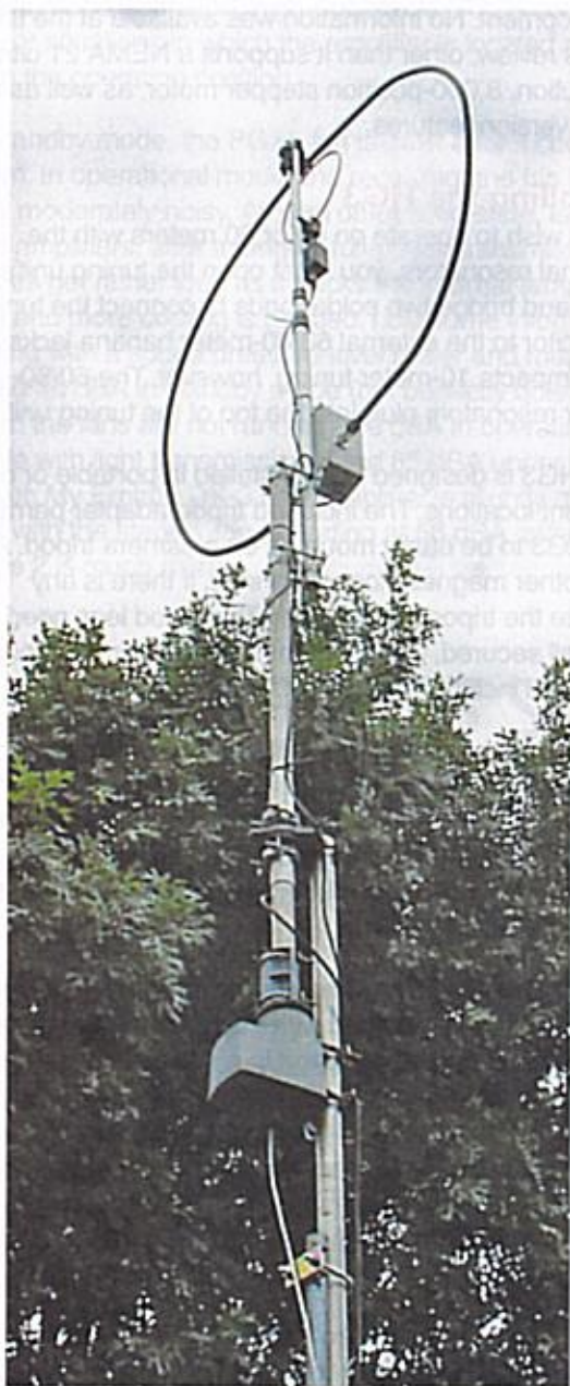
Figure 3 — The HG3 mounted on a pole attached to the author's house and turned with a U105 TV antenna rotator.
