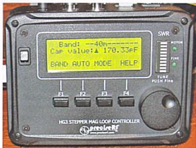
Figure 4 — The HG3 PRO controller with the startup screen shown. The buttons below the screen change function, depending on the screen selected.
