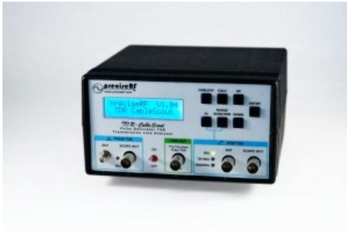
The TDR-CableScout® features isolated high speed samplers and separate device under test (DUT) outputs. This design allows a direct, fast rise time 50 ohm connection to the oscilloscope for accurate TDR measurements without the inconvenience and lower performance “T” connectors with high impedance scope input.
