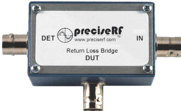
The RLB-I internal reference (three ports) is a high performance Return Loss Bridge optimized for ham radio applications. The internal reference impedance is 50 ohms. The bridge components are precision SMD devices with a wide band 1:1 750 MHz SMD transformer using micro strip construction.
