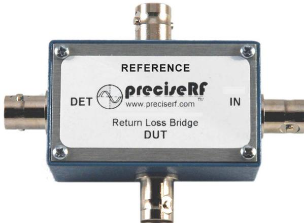
The RLB-E external reference (four ports) is a high performance Return Loss bridge optimized for ham radio applications. The external reference impedance is generally 50 to 300 ohms. The bridge components are precision SMD devices with a wide band 1:1 750 MHz SMD transformer using micro strip construction.
