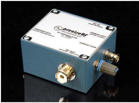
Each SMD Demodulator comes completely assembled in a premium shielded die cast aluminum alloy A380 housing. The housing is blue baked enamel per Federal Standard 595 #25109 over primer wash per DOD-P-15328.
