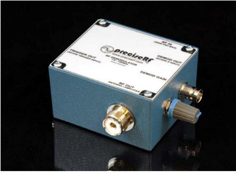
Each SMD-Pro Demodulator comes completely assembled in a premium shielded die cast aluminum alloy A380 housing. The housing is blue baked enamel per Federal Standard 595 #25109 over primer wash per DOD-P-15328.
