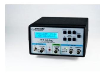
TheTDR-CableScout® features isolated high speed samplers and separate device under test (DUT) outputs. This design allows a direct, fast rise time 50 ohm connection to the oscilloscope for accurate TDR measurements without the inconvenience and lower performance "T" connectors with high impedance scope input.
