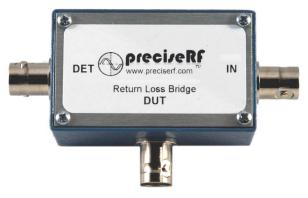
The RLB-I internal reference (three ports) is a high performance Return Loss Bridge optimized for ham radio applications. The internal reference impedance is 50 ohms. The bridge components are precision SMD devices with a wide band 1:1 750 MHz SMD transformer using micro strip construction.
