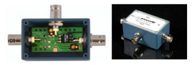
Each RLB-E Return Loss Bridge comes completely assembled in a premium shielded die cast aluminum alloy A380 housing. The housing is blue baked enamel per Federal Standard 595 #25109 over primer wash per DOD-P-15328.
