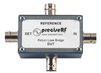
The RLB-E external reference (four ports) is a high performance Return Loss bridge optimized for ham radio applications. The external reference impedance is generally 50 to 300 ohms. The bridge components are precision SMD devices with a wide band 1:1 750 MHz SMD transformer using micro strip construction.
