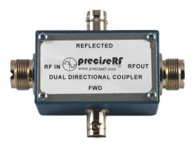
The DDC-1 dual directional coupler measures forward and reflected power of a device in a 50 ohm environment. It is more precise than a simple SWR meter since the reflected and forward power may be observed directly on an oscilloscope.
