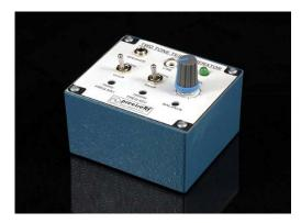
Each TTG1 comes completely assembled in a premium shielded die cast aluminum alloy A380 housing. Each housing is blue baked enamel per Federal Standard 595 #25109 over primer wash per DOD-P-#25109 over primer wash per DOD-P-15328
