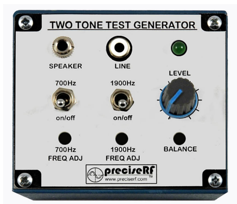
Figure 3 TTG1 Two tone test generator
