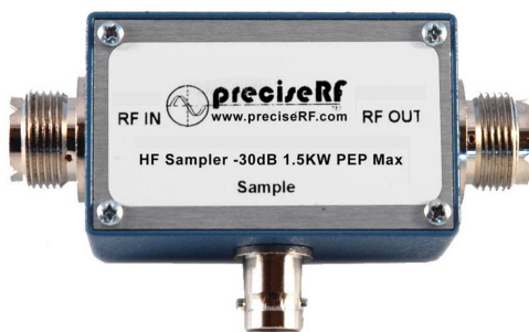
Figure 2 HFS-1.5 HF sampler/coupler -30dB
